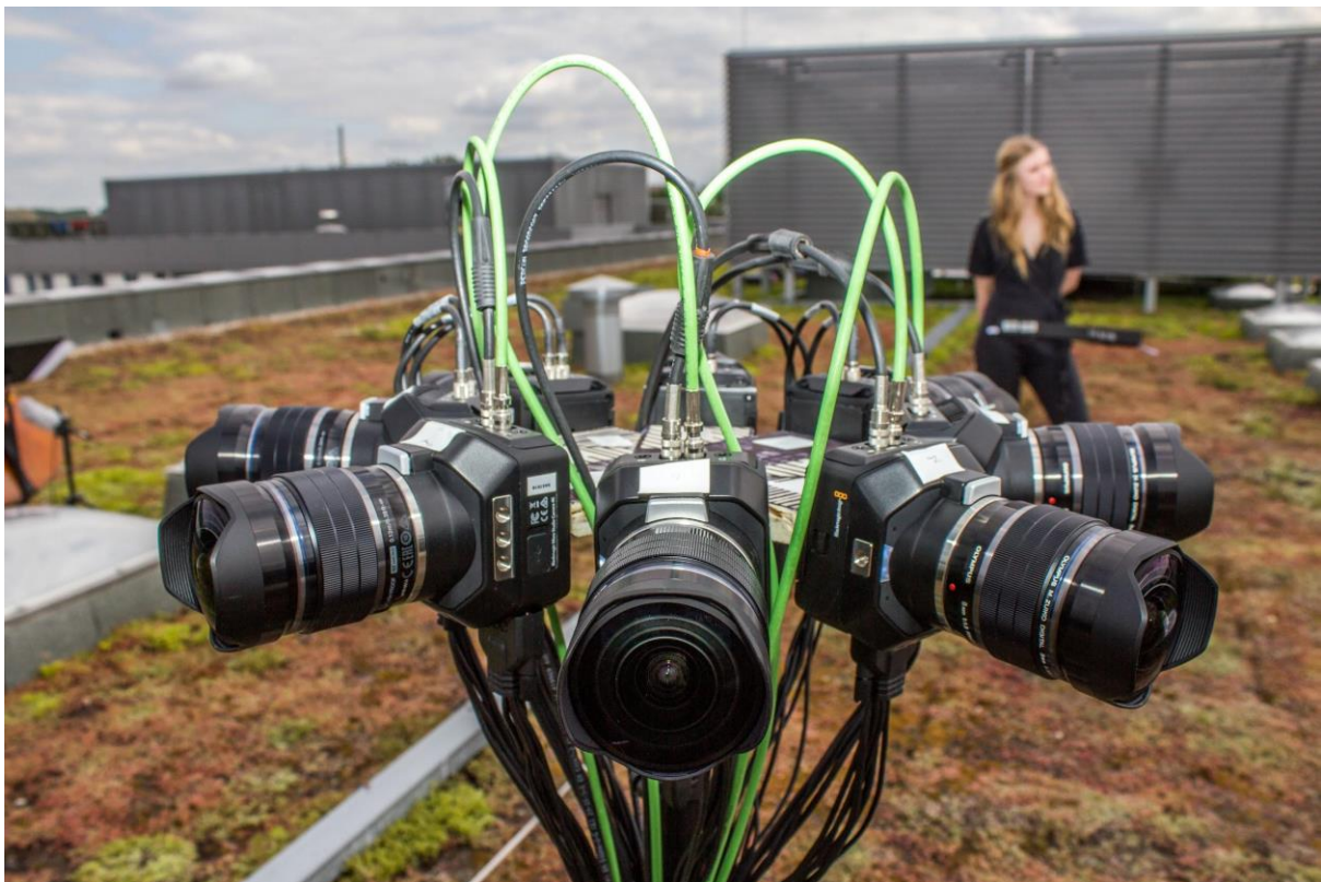
Fig.7 Eight cameras rig for 360 video recordings source: PSNC documentation
