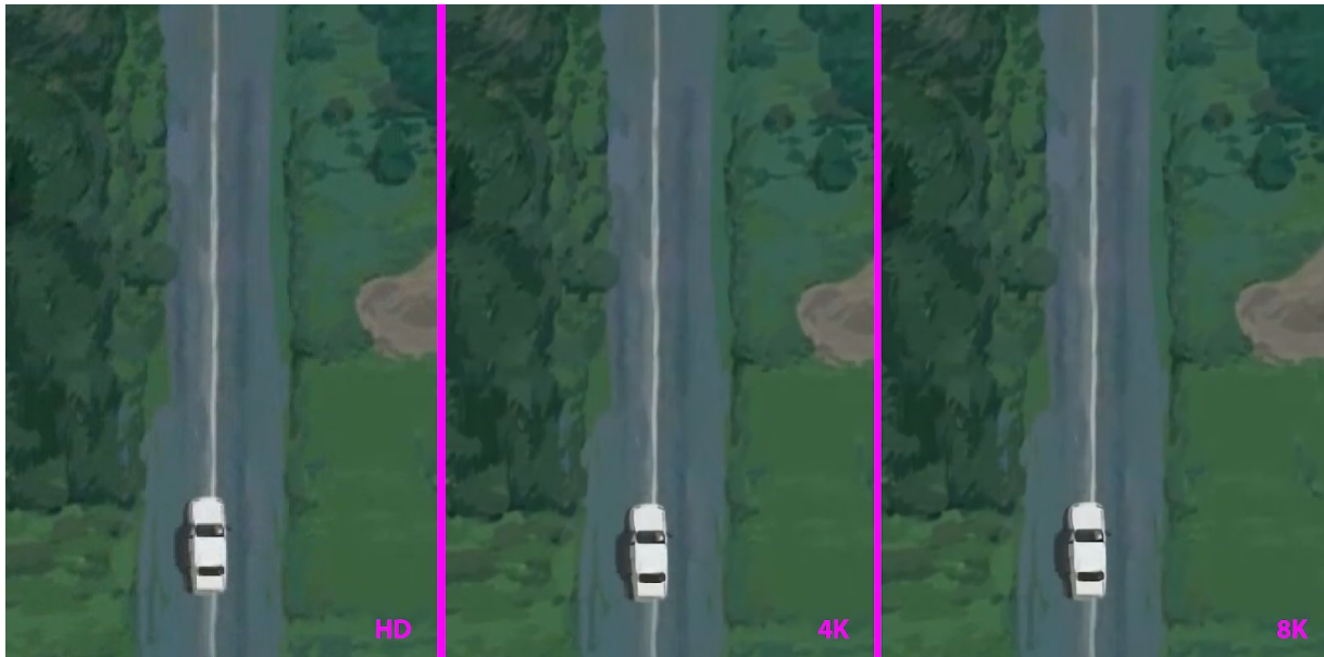
Figure 2. Comparing HD scaled to 400% (nearest neighbor) with 200% 4K upscale & 100% 8K upscale via Waifu2x-caffe (using 2-D illust, CUnet Model, TTA activated, Denoising & Magnifying)
