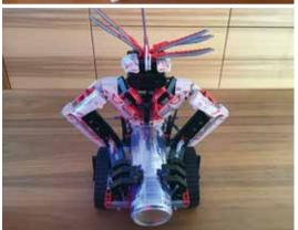
This machine was constructed with gear wheels and a conveyor belt driven by an M-Motor, while the 4-cylinder motor is only a fake motor. To build these machines and devices, I used LEGO technology with seven motors, a remote control, and the robot from LEGO Mindstorms.
