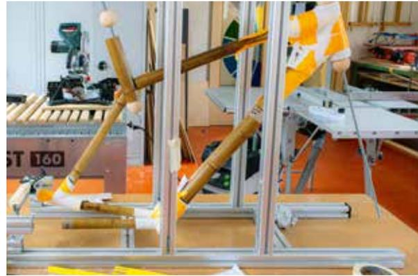
The project *Urban Green: Bamboo Bicycle* deals with the construction of biodegradable bamboo bicycles. But contrary to what one would initially expect, the bamboo-frame structure is simply concealed behind an environmentally friendly image, because synthetic resins and toxic varnishes are used in its construction. The production process itself is also very time-consuming and requires a great deal of manual labor.
